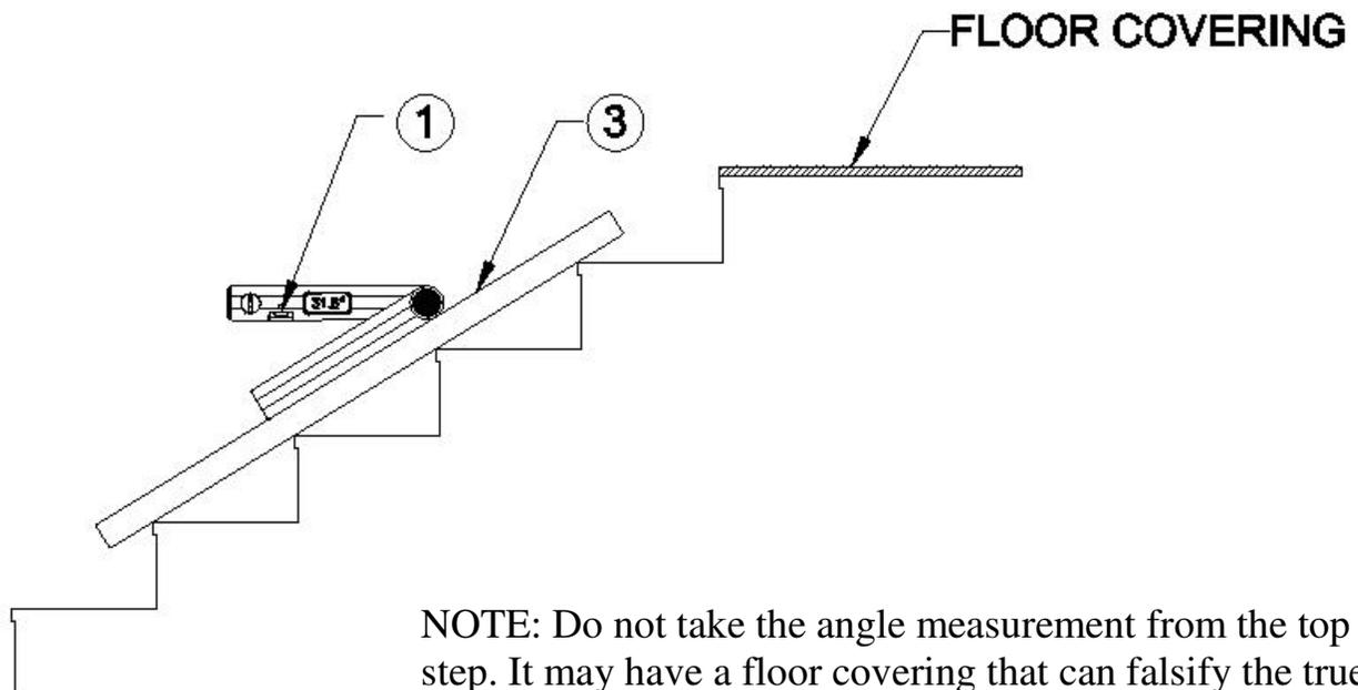
**NOTE:** Do not take the angle measurement from the top step. It may have a floor covering that can falsify the true overall angle of the stairway.
