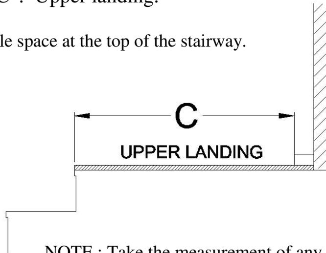
NOTE : Take the measurement of any obstacle that could modify this measure in any way.
